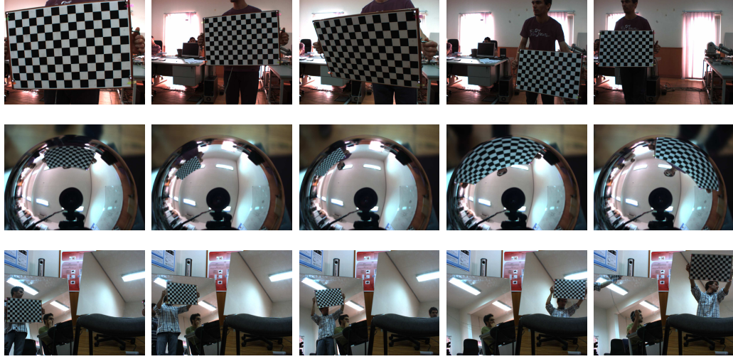
Figure 6.7: In this figure we show five examples of images taken from the chess board used to get the calibration data sets. The first row of images corresponds to the perspective camera; the second row corresponds to the non-central catadioptric camera that uses a spherical mirror; and the last row corresponds to the non-central camera formed by two planar mirrors.
